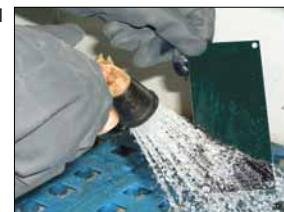
8.2 After the etching process, remove the record-special cliché from the magnetic strips of the extension and rinse the cliché with flowing water.
