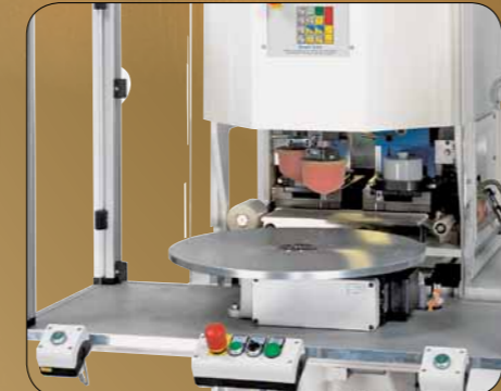
"T2" rotary index table for the feeding of workpieces
