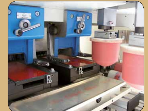
V-DUO with ink residue pick-up system
